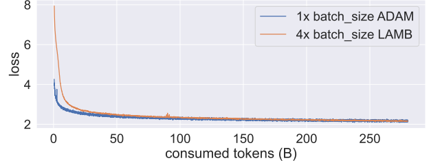
(b) The training loss curve of ADAM optimizer and LAMB optimizer with four times of the batch size.
